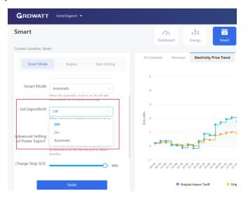
When the Export Limitation Function is selected as Off, the system power will be fed into the grid;
