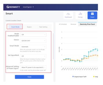
If customers want to set the scheduling plan manually, then can select the [Manual] mode, the export tariff and import tariff threshold could be set separately. The operation interface is as below:
