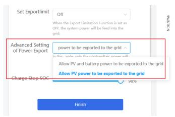
When allow PV and battery power to be exported to the grid, the PV and battery power will be
