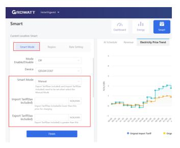
When the Smart Mode is enabled, the system will charge during low electricity price periods, discharge during high electricity price periods, and keep in Load First Mode during other periods.
